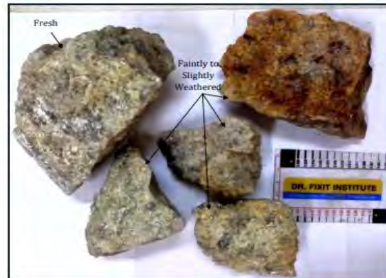
Figure-1: Photograph of fresh and slightly weathered rock particles showing crystalline to granular surface texture.
