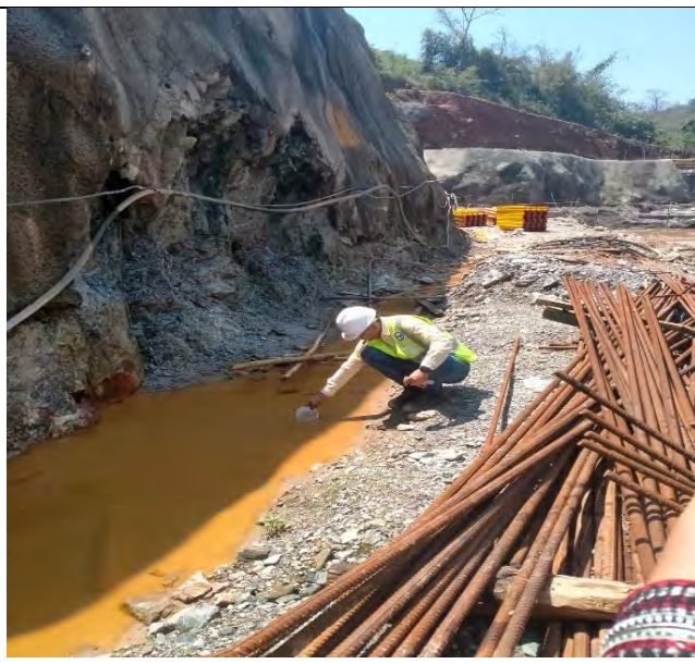
Sample 2 (PH1) from the Pyrite Prone Area at Power House near the side way
